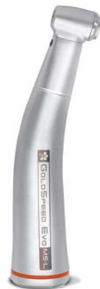
GOLDSPEED Evo M5-L (1:5) Conservative For conservative, prosthetic and general dentistry. Multiplier contra-angle handpiece, gear ratio 1:5, can be heat-disinfected and sterilised in an autoclave, uses \varnothing 1.6 mm FG burs, key-operated bur lock, quadruple spray, ceramic ball bearings, integrated high-intensity, autoclave-safe fibre optic lighting. Head diameter 10 mm.
