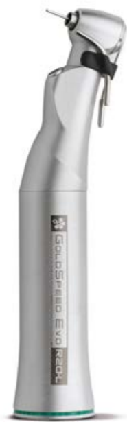
GOLDSPEED Evo R20-L (20:1) Surgical use, Implantology, Osteotomy Specifically for surgical use, gear ratio 20:1, can be heat-disinfected and sterilised in an autoclave, can be disassembled for thorough cleaning, single spray, with hex-type tightening system, for burs and surgical instruments with contra-angle stem \varnothing 2.35 mm, internal Kirschner/Meyer cooling system and external spray, LED with incorporated generator.
