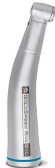
GOLDSPEED Evo S1-L (1:1) Conservative For conservative and general dentistry, gear ratio 1:1, head and handgrip can be heat-disinfected and sterilised in an autoclave, key-operated bur lock, single spray, integrated high-intensity, autoclave-safe fibre optic lighting. Head diameter 9.5 mm.
