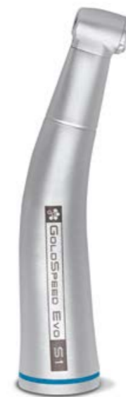
GOLDSPEED Evo S1 (1:1) Conservative For conservative and general dentistry, gear ratio 1:1, head and handgrip can be heat-disinfected and sterilised in an autoclave, key-operated bur lock, single spray. Head diameter 9.5 mm.
