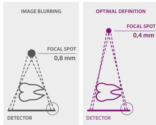
Sharp images at all times RXDC - HyperSphere technology provides your surgery with optimum X-ray quality whatever the type of sensor connected. Now even more powerful, with 70 kV and 8 mA, even more flexible and suitable for all commercially available sensors. The constant potential head tube, associated with the smallest intraoral imaging focal spot available (0.4 mm), ensures the best images whatever your diagnostic needs.
